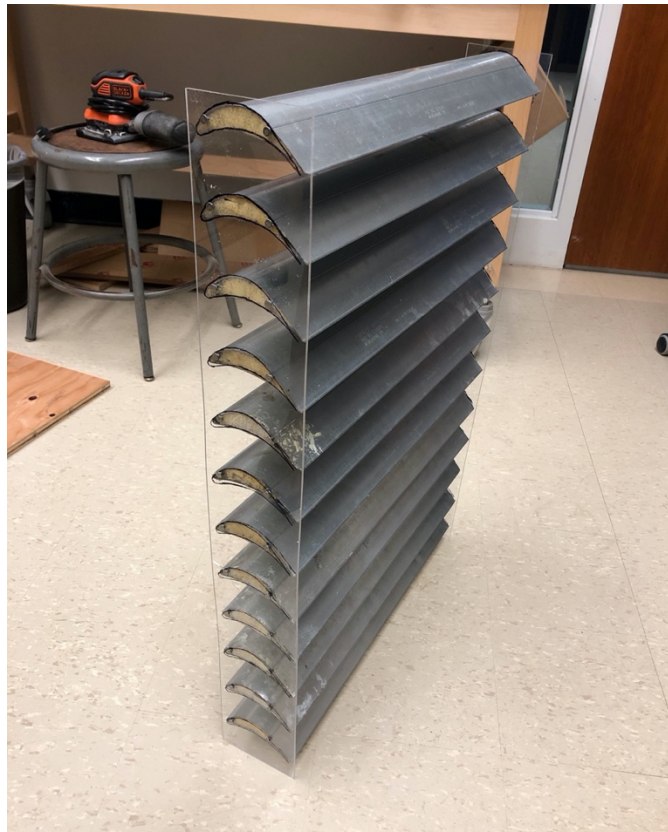
Figure 18. Image of the completed corner vane assembly. Notice the tan-colored foam that fills each corner vane.
