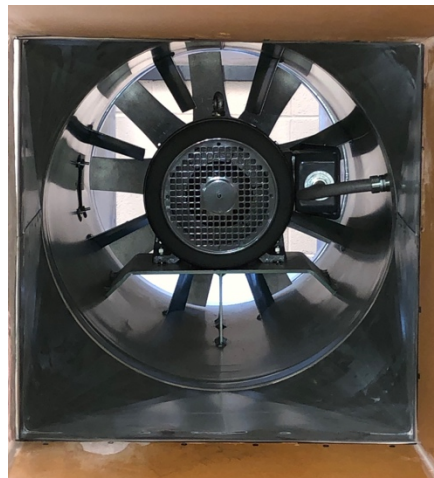
Figure 24. Image of the inside of the motor fan in the Houghton College wind tunnel. This image is taken from a perspective looking upstream through the diffuser towards the fan.
