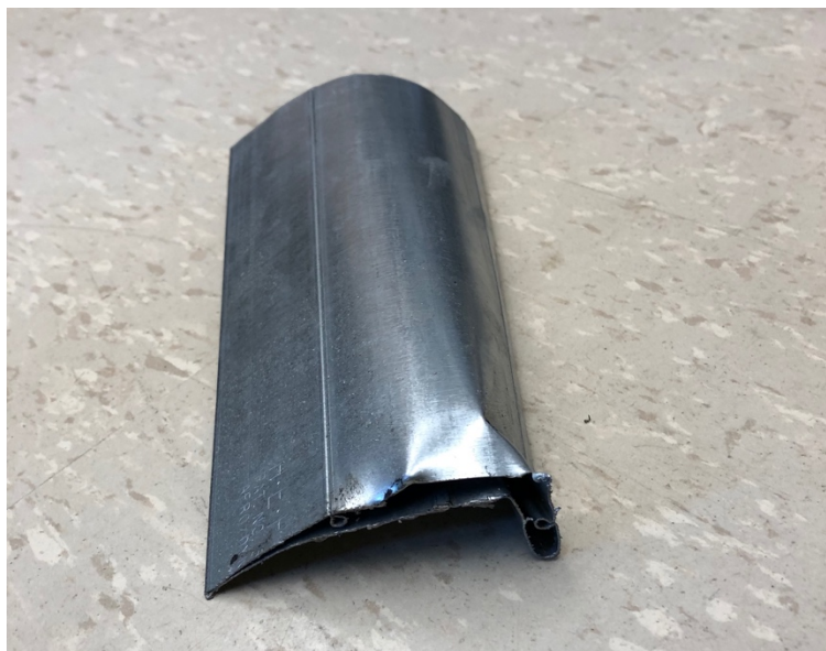
Figure 16. Image of an early attempt cutting the vanes.
