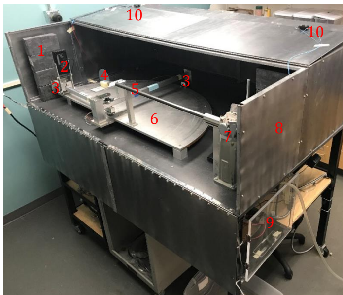
Figure 16. Overview of Houghton XRD. The sample, detector, and x-ray source are mounted on the table, enclosed in steel case. The electronics and water connection are situated below the table.
