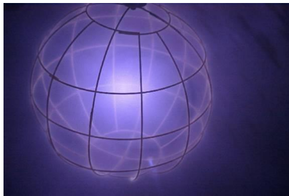
Figure 6. Plasma confined within an IEC device. Using a large voltage on a spherical cathode grid, a large potential well can be created at the center of a vacuum chamber, confining the charged particles that compose the plasma and allowing for fusion to occur. Figure taken from Ref. [23].
