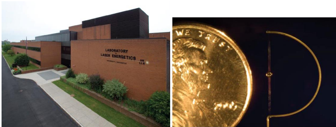
Figure 9. The Laboratory for Laser Energetics and an OMEGA-60 target capsule. (Left) The Laboratory of Laser Energetics (LLE) located in Rochester, NY is the second largest inertial confinement facility in the United States. (Right) Target capsules that are filled with the fusion fuel measure only 1 mm in diameter. Figures taken from Ref. [4]
