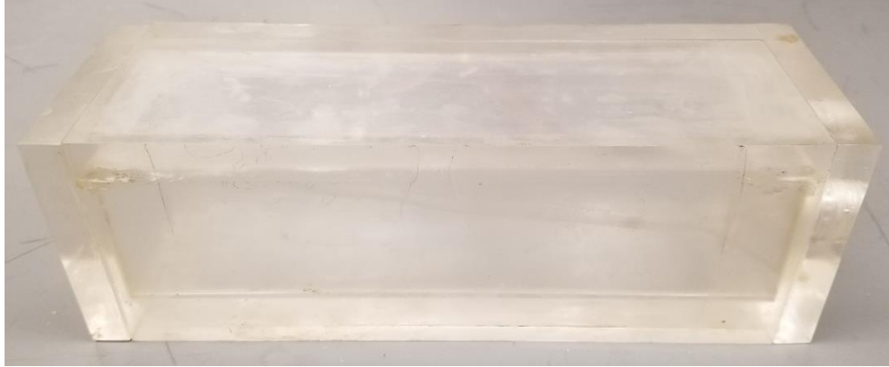
Figure 24. The finished acrylic prototype detector. Many visual imperfections exist within the practice detector: glue joints were not perfectly coupled structurally or optically due to bubbles within the glue joints, measurements of the end caps were slightly off compared to the rest of the body (by about 3 mm), and glue had hardened on the outside surface of the box due to resting on a surface while curing rather than being suspended in a clamp.
