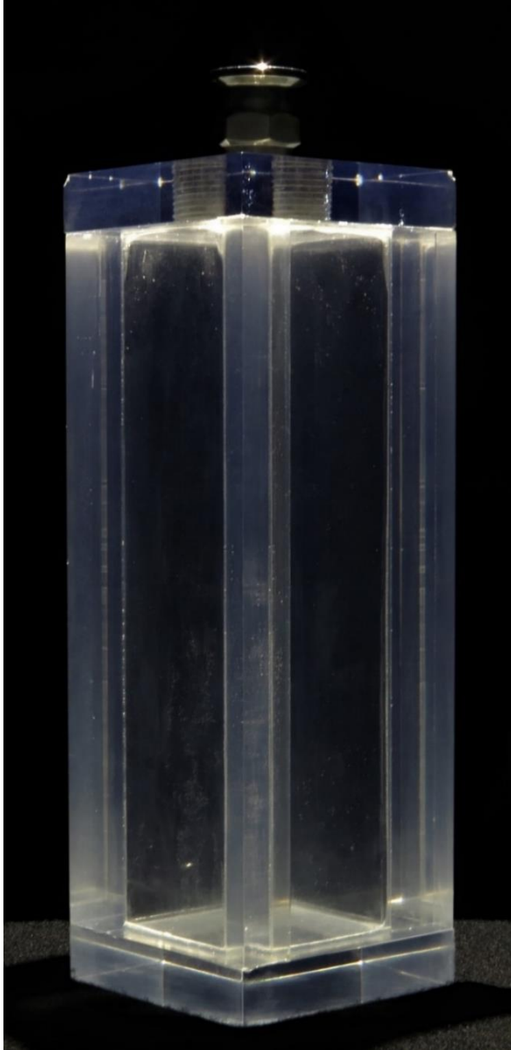
Figure 28. The finished phoswich detector. The second attempt to assemble the detector had only a few visible defects, and all pieces were securely coupled with no visible gaps and few bubbles (all smaller than 1 mm in diameter).
