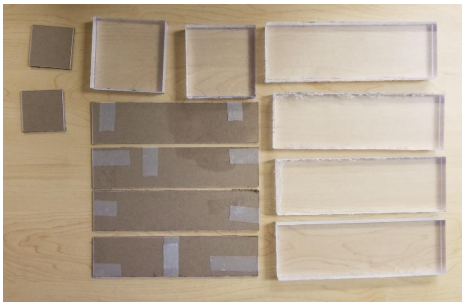
Figure 25. Cut EJ-212 and EJ-240 scintillator pieces. The EJ-212 “thin” scintillator was cardboard-backed (to prevent scratches) while the EJ-240 “thick” scintillator was wrapped in protective, transparent plastic sheet. Both protective measures remained on the scintillator pieces until they were ready for polishing. Referencing Figure 23, pieces labeled 1 are seen on the right, pieces labeled 2 are seen in the center with the cardboard backing, pieces labeled 4 and 5 are seen in the center at the top, and pieces labeled 3 and 6 are seen on the left with the cardboard backing.
