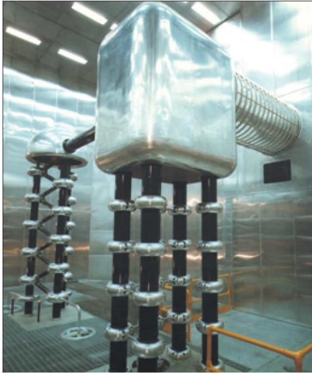
Figure 12. Photograph of one of the Cockcroft-Walton injectors at LANSCE which inject H^+ and H^- ions into the LINAC at 750 keV. Taken from Ref. [16].
