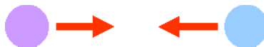
Figure 1. Drawing of a two body interaction. In this example of an attractive, central two body interaction, the force draws the two interacting bodies along the line connecting their centers. However, it is not necessarily the case that a two body interaction be attractive or act centrally.
