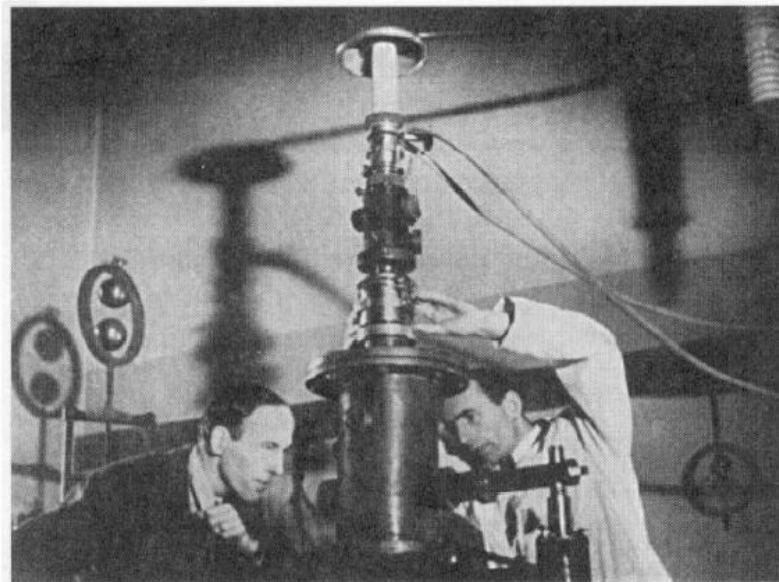
Figure 1.1. The electron microscope built by Ruska and Knoll in Berlin in the early 1930s.
