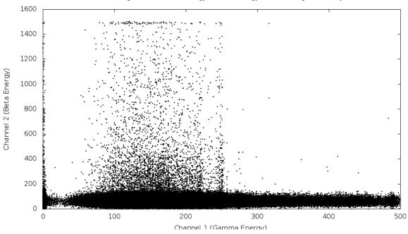
2D Histogram of Gamma Energy vs Beta Energy, Negative Magnet Polarity
