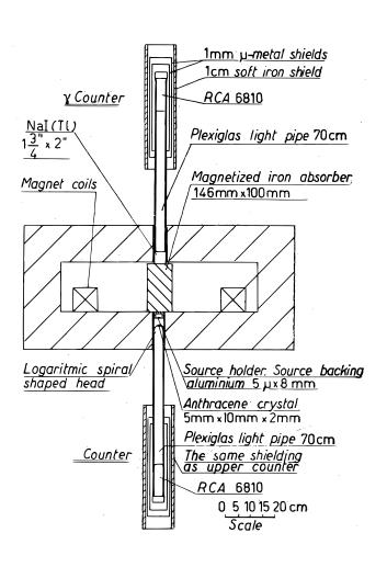
Measured the asymmetry of the circular polarization of the gamma rays
