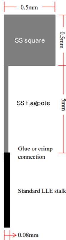
Figure 20. Stainless-steel laser target flag. The deuterated stainless-steel target was attached to a standard LLE stalk. The stalk allowed the target to be held and positioned inside the OMEGA-EP chamber. Figure adapted from Ref [7].
