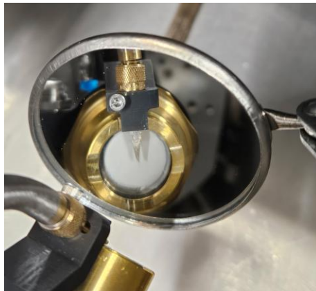
Figure 23. Lithium target on SLICS. A lithium target was placed on the end of SLICS. Deuterons from the sidelighter laser struck the target causing {}^7\text{Li}(d,p){}^8\text{Li} reactions to occur.
