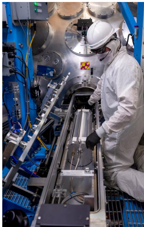
Figure 34. SLICS inside TIM. The assembly allows the SLICS to be extended up to 1.676 m (top). The SLICS inside the TIM while in the retracted position (bottom).
