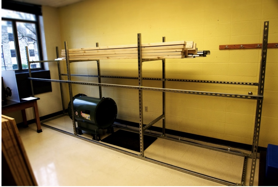
Figure 15. The steel frame constructed out of Unistrut to support the wind tunnel when complete. The acquired vane axial fan from New York Blower is also visible.
