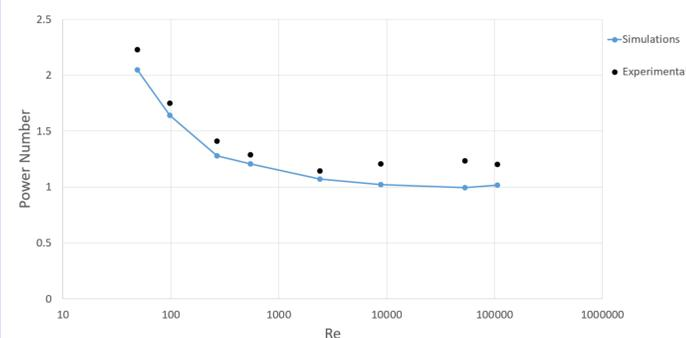
Figure 4: Simulation results compared to SPX Flow experimental data [1].
