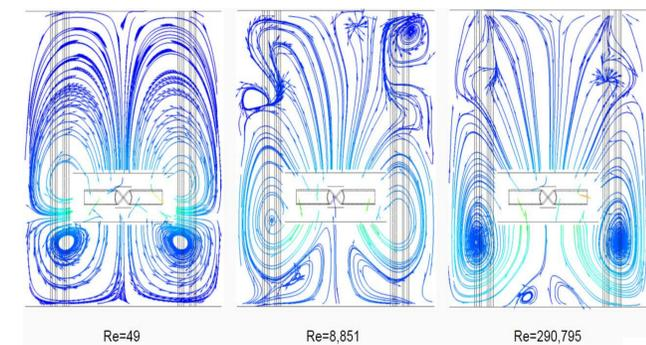
Figure 5: Streamlines constrained to a vertical plane halfway through the fluid domain.
