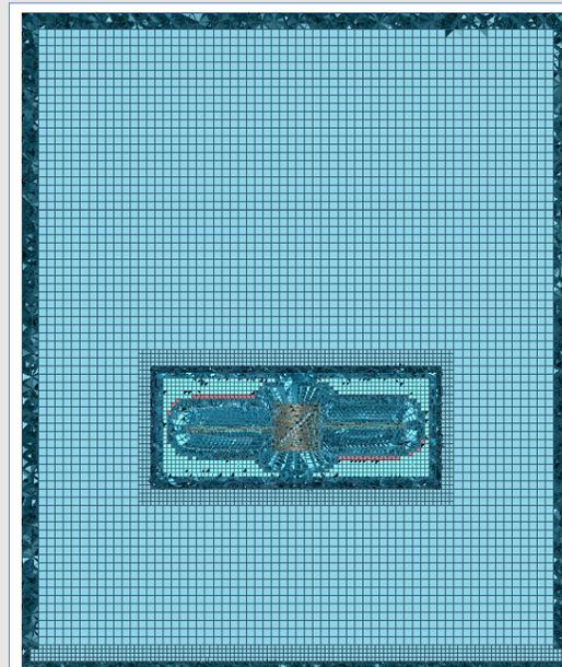
Figure 1: An example of a mesh for CFD. A denser mesh is required in regions where fluid flow is more complex, such as near the impeller and at the boundary layers.
