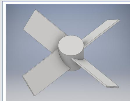
Figure 2: Geometry CAD file of the A200 impeller.
