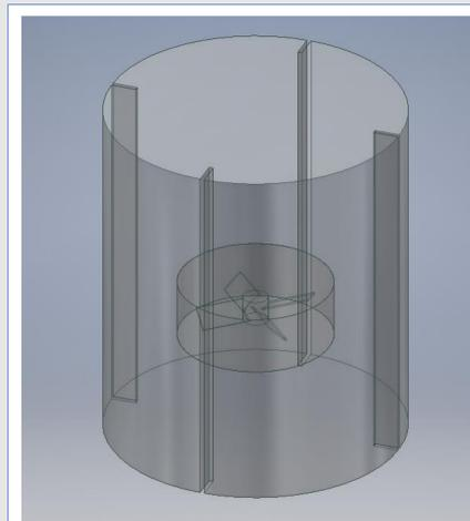
Figure 3: Geometry CAD file of the A200 impeller mixing case. The two "zones" are shown: the cylindrical impeller zone on the inside and the tank zone surrounding it.
