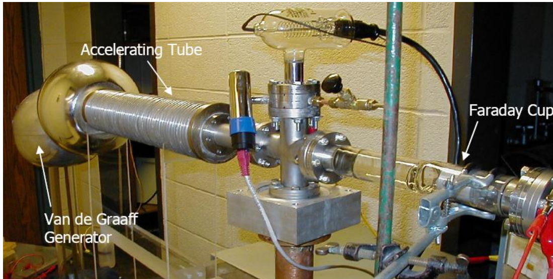
Figure 14. Photograph of the second accelerator tube with the high voltage terminal attached. The accelerator tube was made of alternating aluminum and high-density polyethylene rings. The Van de Graaff generator is located on the left. The supporting base was machined from acrylic. The faraday cup is on the right. The vacuum system is located below the table. Figure taken from Ref. [14].
