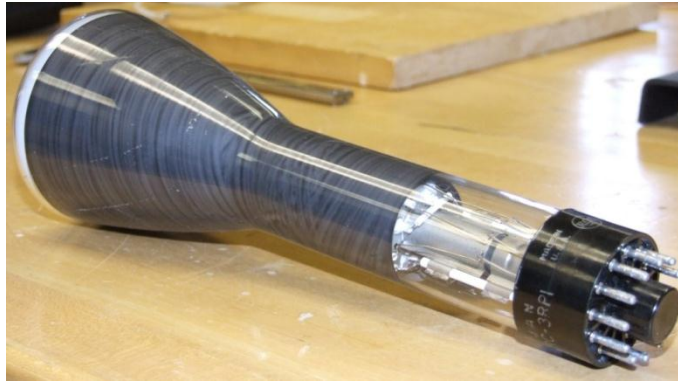
Figure 32. Photograph of the RCA 3RP1 cathode ray tube from which the electron gun and target were taken.
