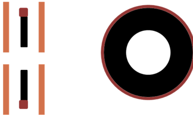
Figure 23. Ring design of the third accelerator tube. The Teflon washers (black) were sealed by Viton o-rings (red) and compressed between two stainless steel washers (orange).
