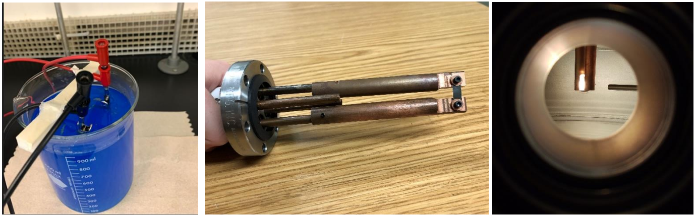
Figure 10. (Left) Copper and tungsten electrodes submerged in \text{CuSO}_4 solution for electroplating. (Center) Vacuum feedthrough used for heating the tungsten ribbon. (Right) Copper plated tungsten ribbon glowing while being heated in the vacuum chamber. Since the ribbon surface is facing in the direction of the getter detector, this photograph is the uncoated back of the ribbon. The end of the collection tube for the turbopump trap is coming in from the right.
