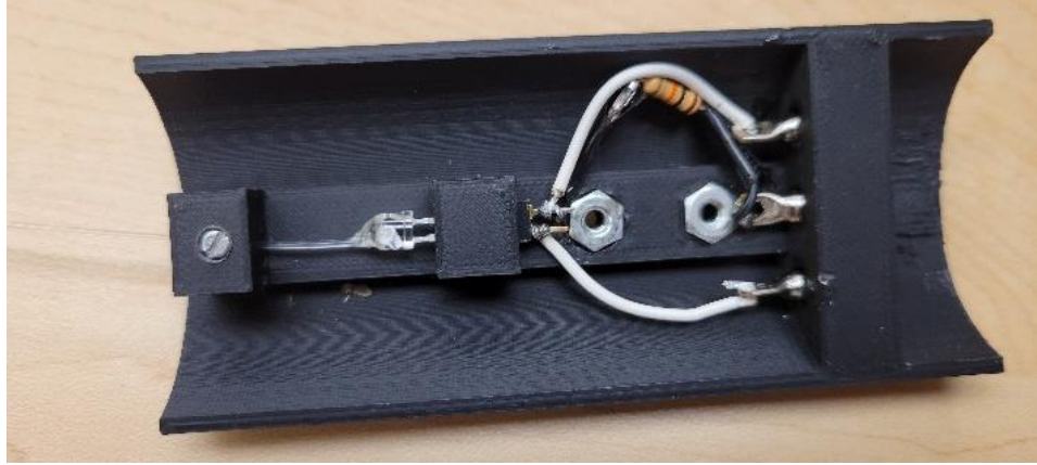
Figure 19. 3D printed phototransistor circuit holder. The set screw, seen on the left, hold the fiber-optic cable in place. A phototransistor attaches to the resistor as well as the inputs for +5V and ground. The third input is the voltage to be measured across the resistor. The two nuts on the right side of the part allow bolts to screw into them so the part can be loosened and slid along a slit in the PVC pipe.
