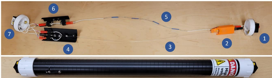
Figure 17. Voltage measurement device innerworkings. The voltage divider and phototransistor circuits are contained within a PVC pipe. The input terminals are attached to the PVC cap shown at 1 which connect to a 3D printed part, 2, that holds the LED light and fiber-optic cable, 3, as well as the resistor chain, 5. Both the phototransistor circuit holder, 4, and the voltage divider circuit holder, 6, can be adjusted within the PVC pipe to keep the fiber-optic cable and resistor chain extended within the pipe. The circuit is accessed through banana connectors attached to the PVC cap at 7.
