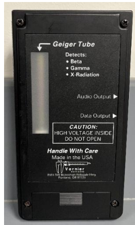
Figure 17. Geiger Tube Detector. A battery powered Geiger tube capable of detecting beta, gamma, and x-ray radiation can send the number counts via electric pulses.
