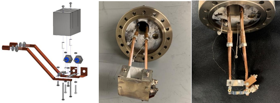
Figure 6. In the exploded drawing of the evaporator (left) a diode circuit controlled which boat is heated. First, one diode allowed current to flow one direction through a stainless-steel boat to heat and evaporate a lithium metal pellet, then another diode allowed current to flow the opposite direction, heating a molybdenum boat to evaporate a tin pellet. A stainless steel “house” surrounded the boats in order to keep the metal, as much as possible, from depositing on the diodes, feedthroughs, and vacuum chamber walls. A photograph (center) of the evaporator with the “house” and with the “house” removed (right) to reveal the boats and diode.
