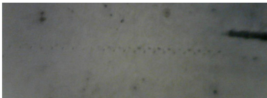
Figure 10. Micrograph of the tin surface after being in the profilometer. A series of small pinholes is visible where the probe touched the tin surface.
