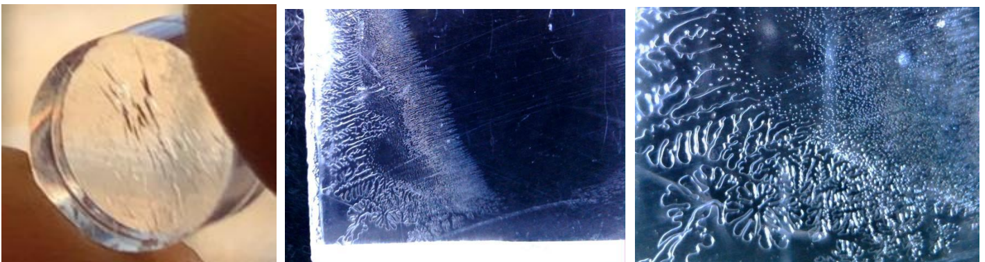
Figure 14. (Left) Photograph of the small phoswich detector that was sent to LLE to test for outgassing. After the detector was removed from the vacuum, small cracks were discovered. (Center and Right) Photographs of phoswich detector after removing it from the test vacuum chamber at Houghton University for a detector that was glued with epoxy that had air in it.
