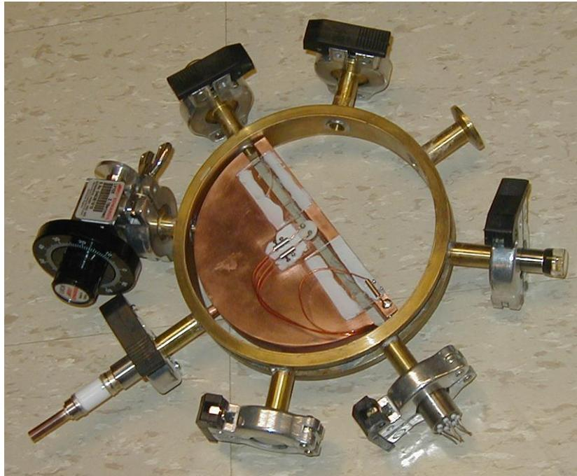
**Figure 27.** A photograph of the electrode assembly. The copper dee is held to the dummy dee with three glass microscope slides glued in place with vacuum epoxy. The grounding wire can be seen on the dee, as well as the feed-throughs. The filament is held in place with short wires soldered to the contacts and barrel connectors, held to the dee with epoxy and insulated by a microscope cover slip.
