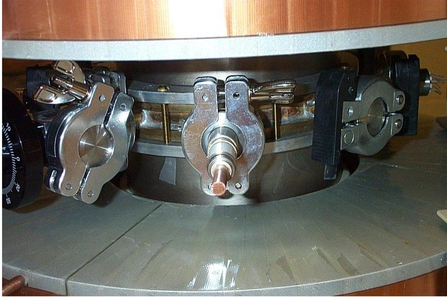
**Figure 25.** A photograph of the vacuum chamber situated between the magnet pole faces. The ring is made of a strip of brass and two outer rings to which the strip is soldered, and eight quick flanges that are soldered in place around the ring. Two aluminum plates equipped with O-rings are screwed together around the ring to form a vacuum tight seal. The device is centered between the pole faces of the magnet.
