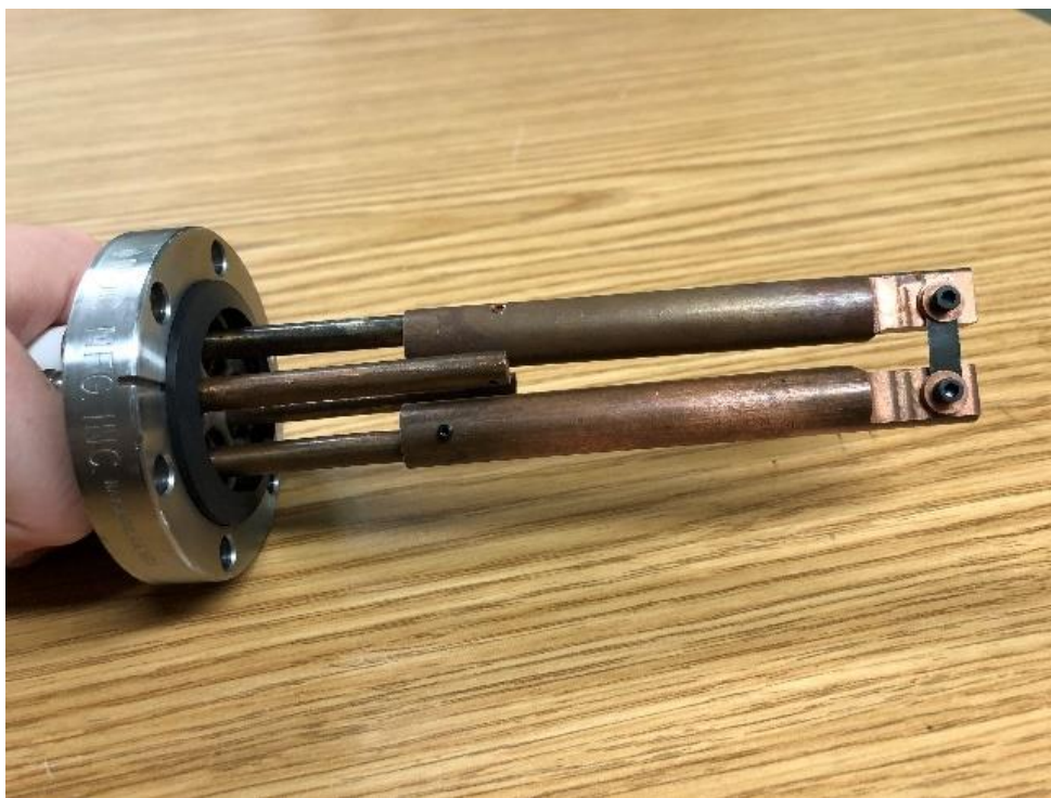
Figure 15. Exploding wire device with tungsten ribbon target. Four copper rods pass through the conflat electrical feedthrough with two larger copper extenders able to hold the tungsten ribbon in the center of the test chamber. The tungsten ribbon may face either the getter system or the turbopump system by detaching the copper extenders, rotating them 90 degrees, and reattaching them to the other two copper rods.
