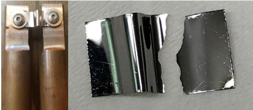
Figure 35. Tungsten ribbons after exploding wire experiments. No macroscopic amounts of copper could be seen on the post-explosion tungsten ribbons, as supported by results from the rotating shield experiment.
