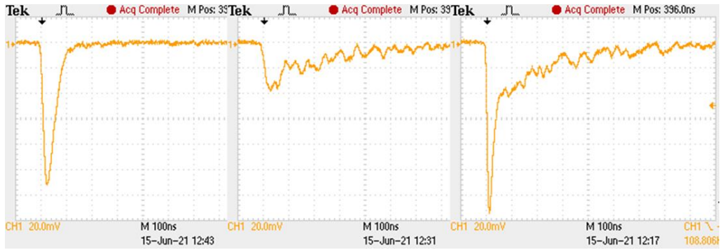
Figure 20. Possible pulse shapes from a phoswich detector. A ^{207}\text{Bi} source, emitting a spectrum of beta particles as well as 1 MeV and 0.5 MeV monoenergetic beta particles, was used to produce the pulses, which were viewed on a Tektronix TDS 2024B oscilloscope. The left pulse was from the dE detector, the middle pulse was from the E detector, and the right pulse was from both detectors.
