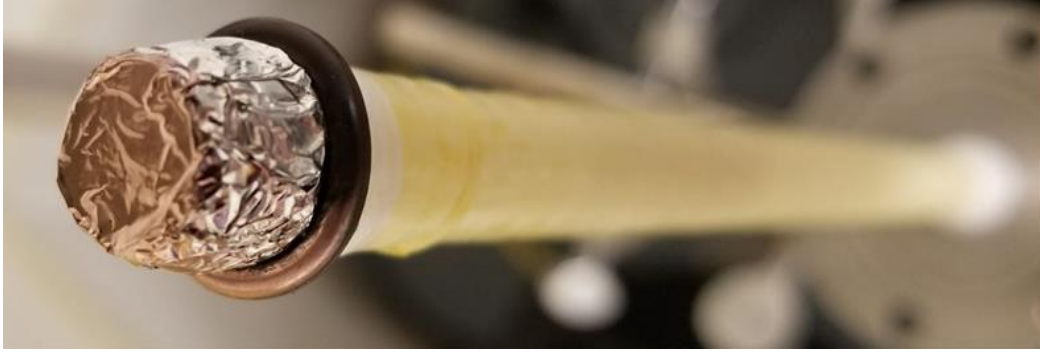
Figure 31. Copper evaporated onto getter foil. This photograph, taken after several exploding wire experiments, showed that the evaporated copper had been successfully trapped by the getter foil.
