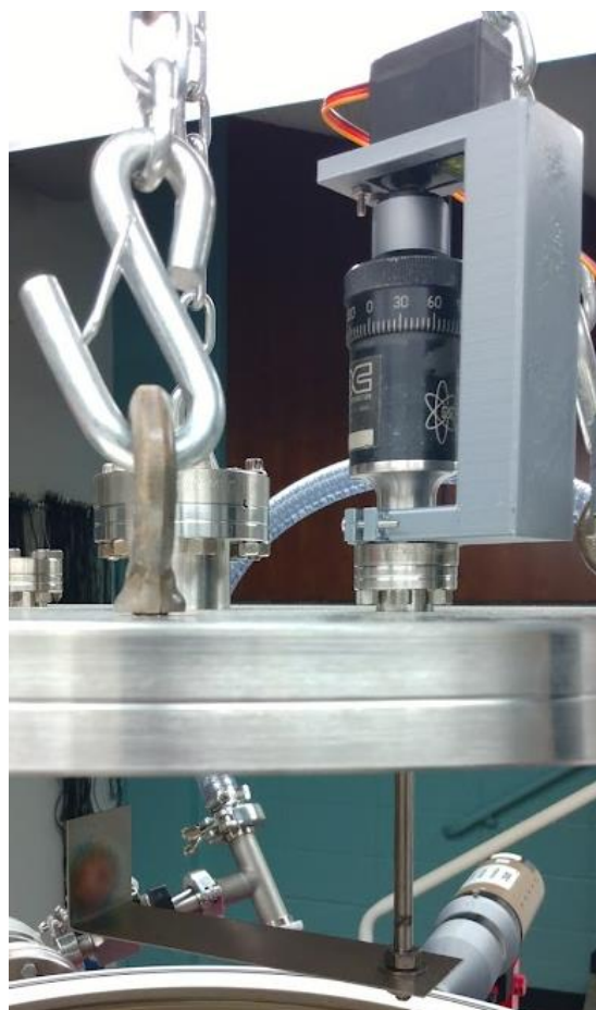
Figure 18. Rotating shield with servo motor. The 0.92 mm thick aluminum shield formed a 14.1 cm by 4.2 cm “L” shape. The shield was attached to the test chamber lid with a rotary feedthrough, and a servo motor was mounted with 3-D printed plastic parts to rotate the shield. The shield blocked the inside of the test chamber’s turbopump port in its default position, and could rotate 120 degrees to rest between the getter detector and the target.
