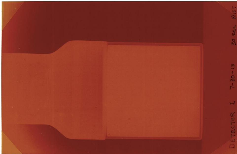
Figure 27. X-ray scan of Detector I exposed for 30 seconds at NIST, used to find a 2.5 mm gap between the crystal and face of the detector which was simulated as BaO, bringing the GEANT simulation into agreement with experimental measurement.
