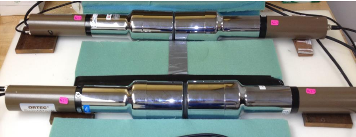
Figure 4. Counting station at the Ohio University Experiment in 2013. This setup was used to measure ^{11}\text{C} beta-decay in the carbon and polyethylene disks by detecting, in coincidence, 511 keV gamma rays released by positron annihilation.
