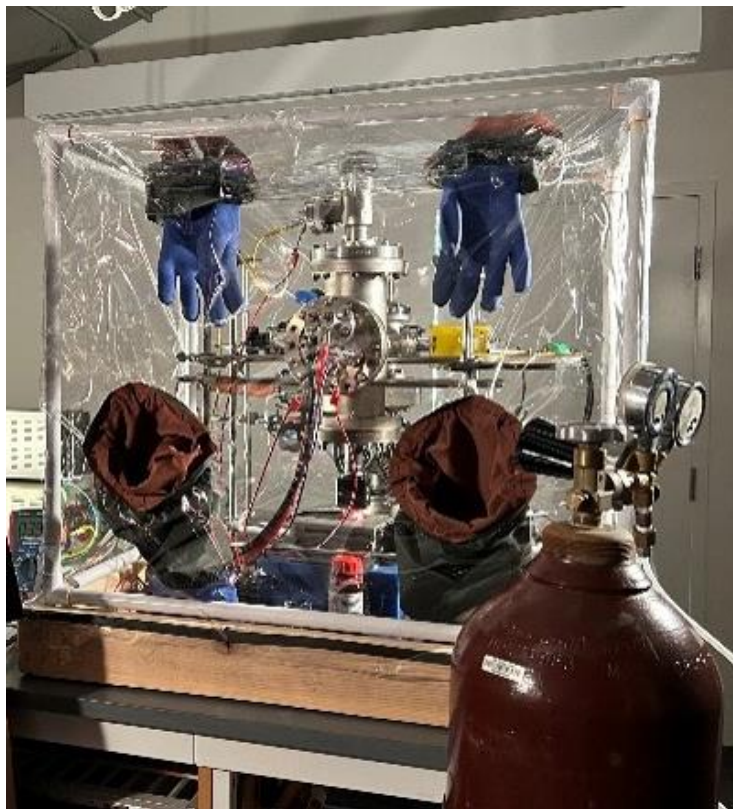
Figure 22. Photograph of the lithium deposition chamber. The glove box was filled with argon to prevent oxidation of the lithium in air. Two pairs of gloves were accessible from the outside of the glove box for handling at multiple heights. The two leads of the power supply were connected to the copper electrodes on the face of the deposition chamber.
