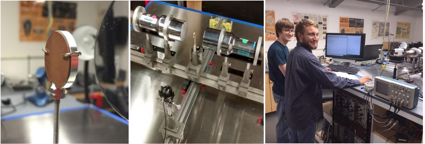
Figure 8. The ^{68}\text{Ge} source assembly (left) and the source assembly placed between the two NaI detectors (center). The camera is used for precisely positioning the detectors relative to the active region on the source. NIM and CAMAC electronics process and digitize the detector pulses which are read out into the computer (right).
