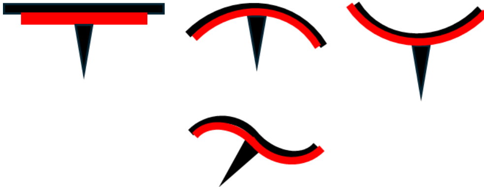
Figure 13. Piezoelectric buzzer actuator. The red piezoelectric ceramic is bonded to a black metal disc. When a voltage is applied, the ceramic changes its lateral dimensions, causing the combined structure to bend. This bending motion displaces the tip (triangle), allowing precise control of position.
