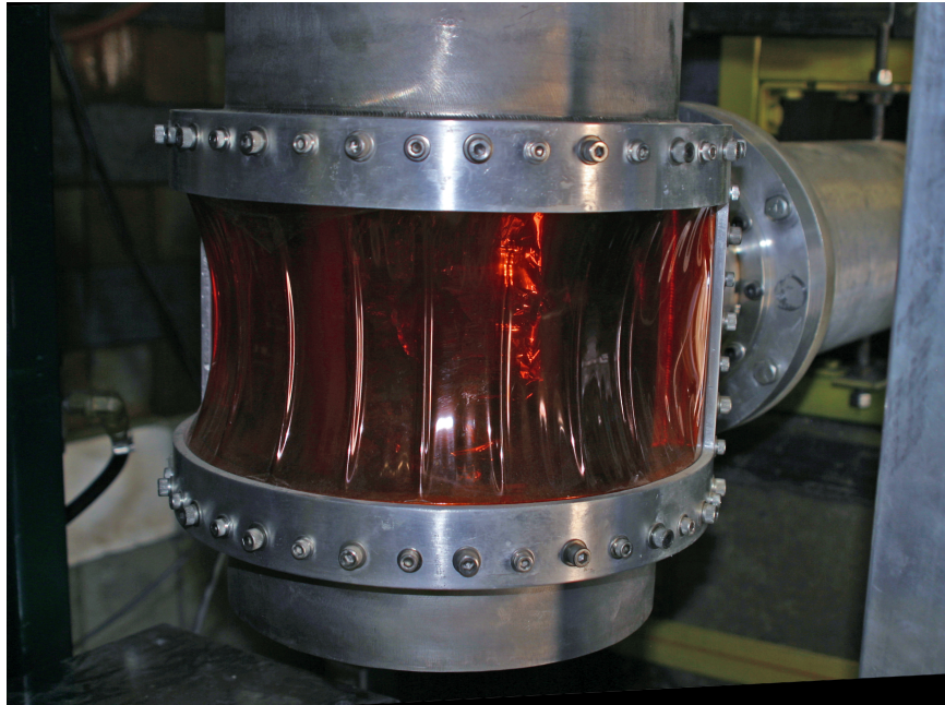
Figure 2.10 Photo of the deuterium target chamber. The deuterium target was contained in a vacuum chamber with orange kapton windows. The beam pipe is attached to the chamber at right in the photograph.
