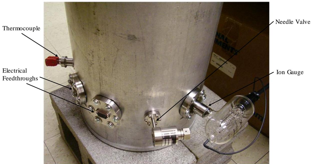
Figure 33. View of installed feedthroughs at bottom of deposition chamber.
