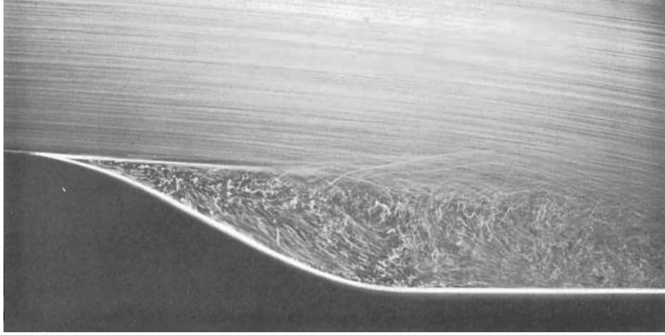
Figure 11. Image of separation of a laminar boundary layer. Water flows over a surface that becomes convex. Air bubbles in the water show that this causes the flow to separate from the surface. Figure taken from Ref. [21].
