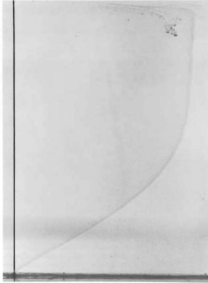
Figure 10. Image of laminar boundary-layer profile. The fluid is flowing from left to right. The black line at the left of the image is a tellurium wire that causes a colloidal column to form in the fluid when an electric pulse is applied to it. The curved dark line in the image is a colloidal column of particles that have been swept downstream by the motion of the fluid. Figure taken from Ref. [21].
