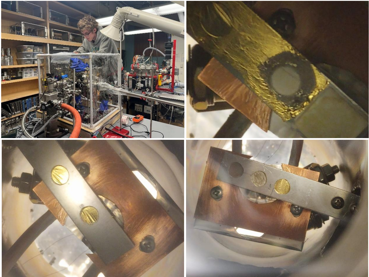
Figure 6. (Top left) Houghton University student Andrew Bo preparing the deposition chamber to make a thin Lithium target film. (Top right) A thin film of lithium (gray) was deposited on the self-supporting 116 nm thick gold foil. (Bottom left) From the RBS data it was clear that the gold and lithium mixed. In this photograph, lithium was deposited opposite the side shown, and the mixing did not reach the back surface of the gold, which remained gold colored. (Bottom right) In this photograph, the lithium penetrated all the way to the back surface of the gold. The target frame has three openings, the leftmost is a quartz viewer, the center is lithium coated gold, and the rightmost is bare gold.
