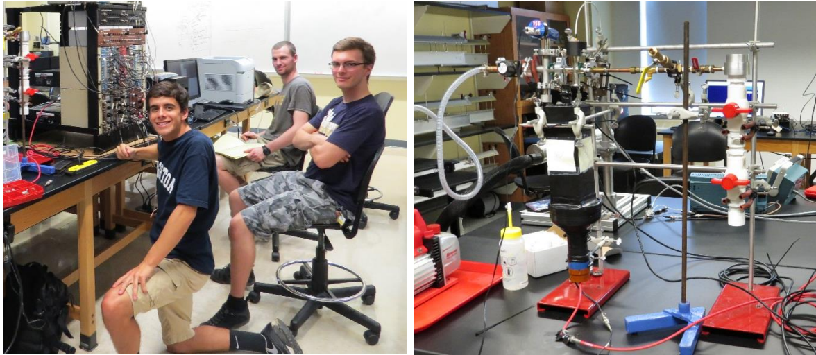
Figure 12. Experiment setup. (Left) Houghton students (left to right) Salvatore Ferri, Steven Raymond, and Tyler Kowalewski assembling the detector system at SUNY Geneseo. (Right) The ^{41}\text{Ar} is prepared in the white PVC gas cell at the right of the photograph. Air is removed from the transfer line and the detector by the rotary pump, then the valve will allow the argon to enter the black detector on the left side which will count ^{41}\text{Ar} decays.
