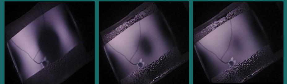
**Figure 4.** A phenomenon was observed through the bottom window (Fig. 1) while the lithium pellets were heating up in the boat (Fig. 3). As the lithium melted, it formed a cool dark spot on the boat (left). As the boat temperature stayed near  $400\text{ }^{\circ}\text{C}$  this dark spot slowly disappeared (center and right). This recurring process shows the evaporation of lithium over time. As the area of the dark spot fades completely, the lithium is all evaporated.
