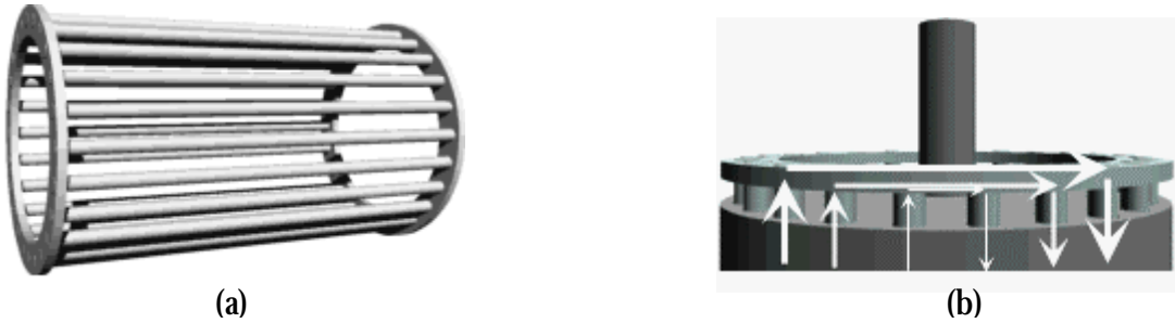
Figure 7. Cage Rotor. The cage rotor of induction generators contain conducting bars (a) are commonly made of copper or aluminum connected electrically by aluminum end rings so that current (shown with white arrows) can be induced through the bars (b). Figure taken from Ref. [11].
