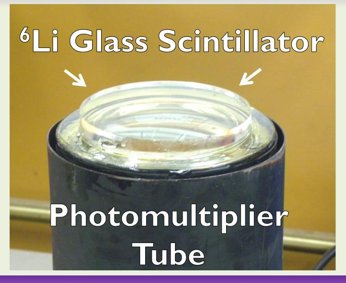
Detects neutron from exothermal reaction:
