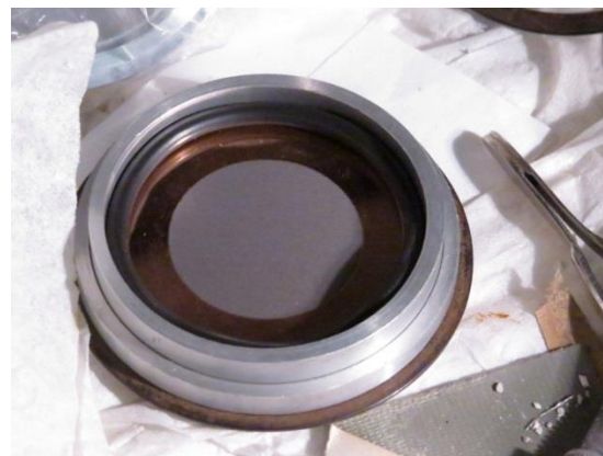
Figure 3. The tritium tritide target prior to insertion into the beam.
