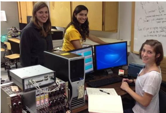
Figure 9. Three counting stations were used for the graphite target, the polyethylene target, and the graphite shields. Positron annihilation gamma rays detected in coincidence were digitized and recorded using an MPA-4 multiparameter system.
