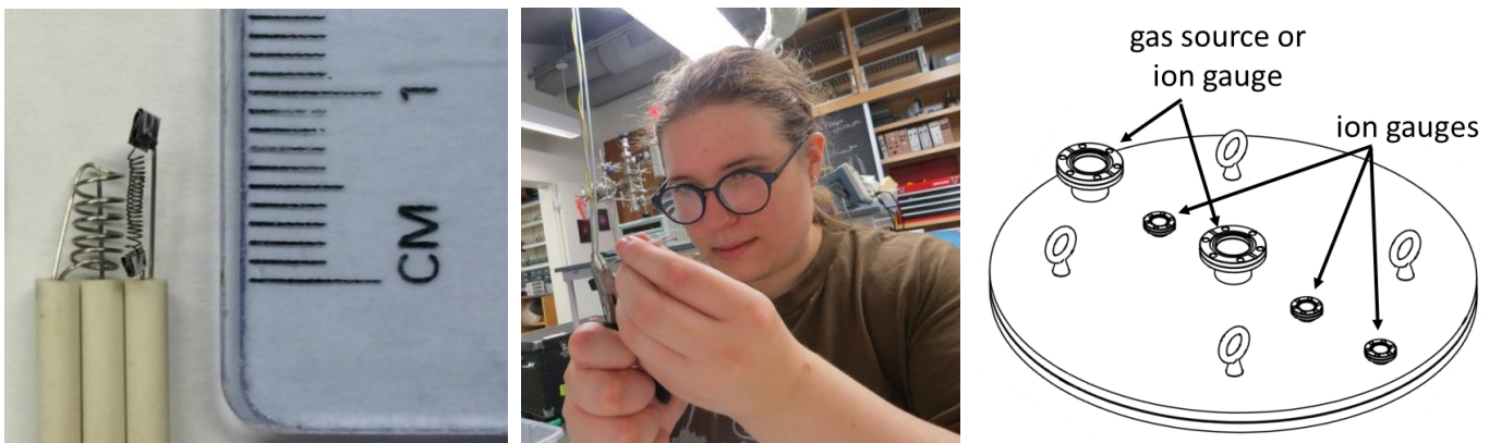
Figure 6. (Left) The high speed ionization gauge. The filament is the smaller winding, the grid is the larger winding which is coaxial with the collector wire. (Center) Houghton student Emma Bruce needs steady hands to carefully clip the leads on the ion gauge she has just completed. (Right) A new vacuum chamber lid will have ports for inserting these ion gauges, as well as gas sources, to measure the motion of gas in the chamber.
