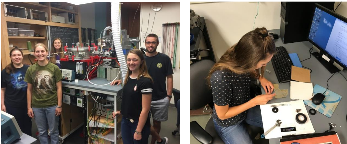
Figure 16. (Left) Houghton and SUNY Geneseo students working together on the test experiment. (Right) Houghton Student Katelyn Cook used a 3D printer to make a light tight housing for the silicon detector, and is shown here installing the thin foil window that allows the beta particles to enter the detector.
