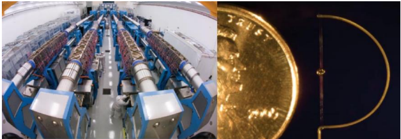
Figure 4. OMEGA Laser bay at LLE and an ICF target. The laser bay (left) consists of preamplifiers, amplifiers, calorimeters and spatial spacers to get the desired wavelength and energy of the laser beams to then focus on the target in the chamber. The ICF target (right) is compared to the size of a penny. This target is about 1 mm in diameter. Figure taken from Ref. [7].
