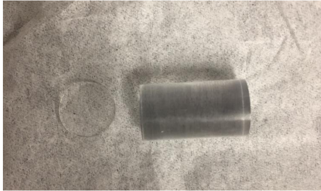
Figure 30. Plastic Scintillator Detectors. (Left) dE detector Eljen EJ-200 1 mm thick with 2.1 ns decay time. (Right) E detector Eljen EJ-204 18 mm thick with 285 ns decay time.
