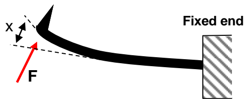
Figure 3. A cantilever with a tip at one end and fixed at the other end. The displacement x of the end of the lever is directly proportional to the force on the tip.
