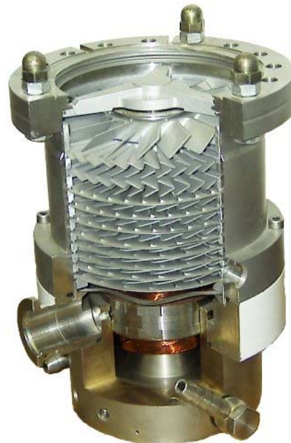
Figure 13: A cutaway of a common turbomolecular pump showing the change in blade size as progressing through the apparatus. Figure taken from Ref. [22].
