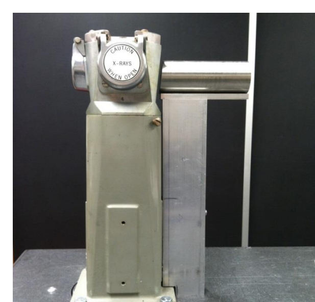
Figure 4 (left)- pictured is the Phillips-Norelco X-ray source. The target in the diffraction tubes is copper. The cylinder in front of the X-ray sources is a steel collimator with a \frac{1}{4} " hole drilled down the center.
