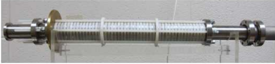
Figure 32. Photograph of assembled accelerating tube. The high voltage terminal mates to the large brass disc at left.
