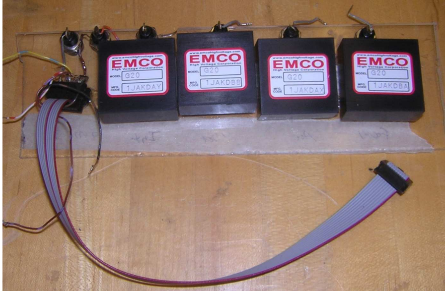
Figure 48. Photograph of HVDC converter Plexiglas mount board. Each HVDC converter powers a different section of the electron gun. Signal from the transistor amplifier is supplied via a ribbon cable. The HVDC connects to the electron gun via banana cables.
