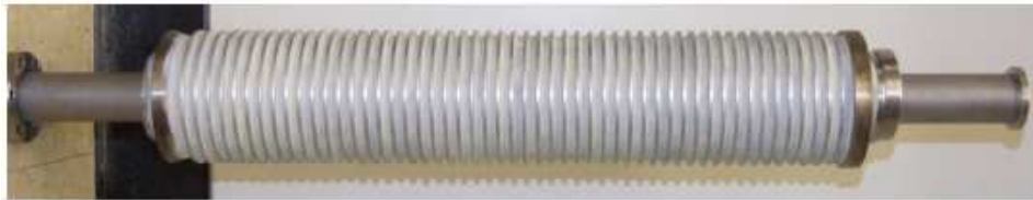
Figure 24. Photograph of accelerator tube. The electron gun mounts to the left. The brass flange on the left is machined to mate with the high voltage terminal.
