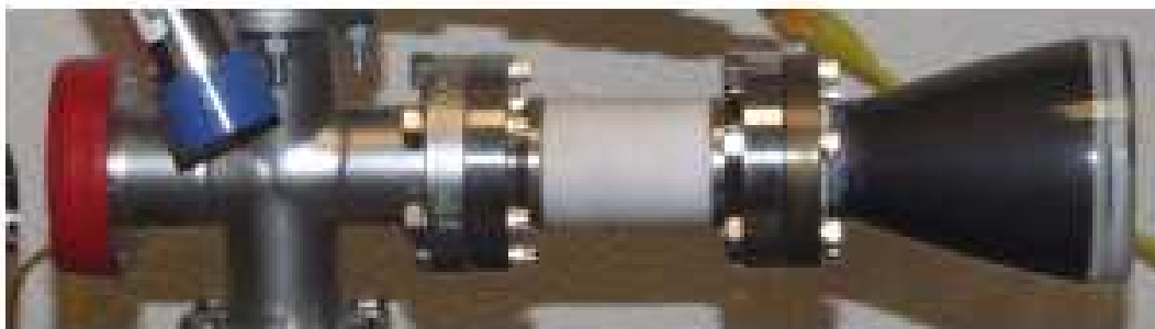
Figure 34. Picture of phosphorescent screen. The white ceramic tube electrically isolates the screen from the grounded vacuum system at left.
