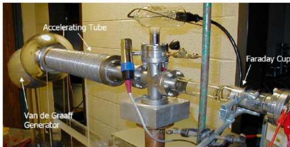
Figure 27. Photograph of accelerator. Electrons are accelerated from left to right down the accelerating tube. The Van de Graaff generator is used to generate the high voltage. The faraday cup measures the beam current. Taken from Ref. [45].
