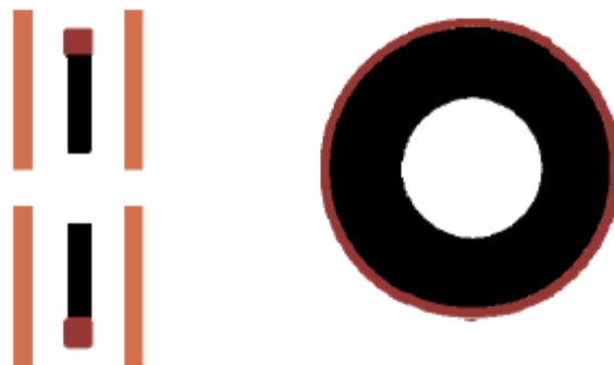
Figure 30. Drawing of ring stacking. Teflon rings (black) were sealed by Viton O-rings (red) and compressed between stainless steel washers (orange). Taken from Ref. [46].
