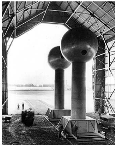
Figure 9. Picture of Round Hill generators. They generated a potential of 5.1 MV. Taken from Ref. [26].
