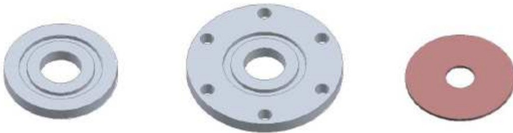
Figure 31. 3D rendering of rings. The standard polyethylene ring is at the left, the polyethylene ring with threaded rod guides is at center, and the stainless steel washer is at left. Taken from Ref. [46].
