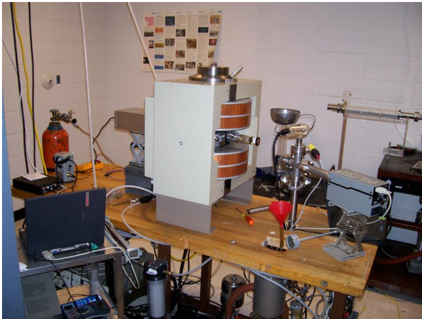
Figure 13. A photograph of the Houghton College Cyclotron. The electromagnet is prominent in the picture, with the chamber between the poles. The vacuum system is below the table on the right. Underneath the table on the left is the equipment for the RF system. The helium tank is also visible.
