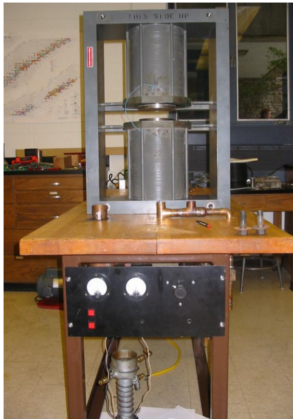
[Figure 4.1] A photograph of the current status with magnet, control panel, and nearly a completed vacuum system.
