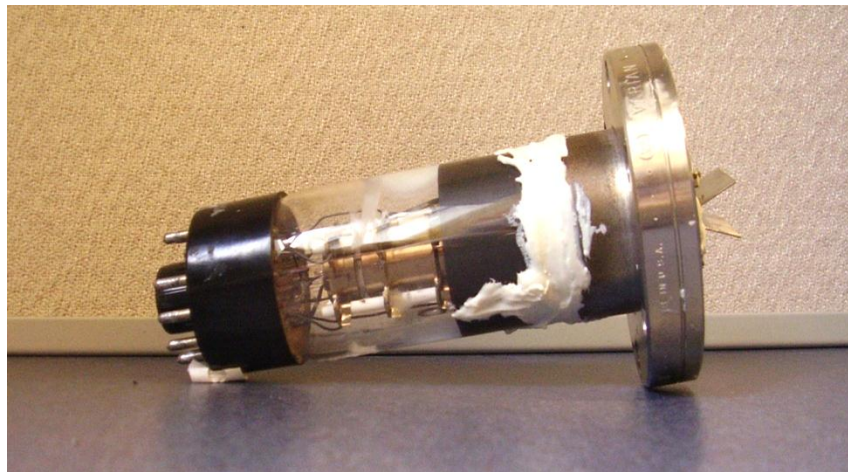
Figure 15. Current electron gun. The last two deflection plates can be seen protruding from the flange. The vacuum epoxy is visible where the flange and electron gun are connected. This electron gun includes the filament, cathode, accelerating grid, focusing grid and deflection plates.
