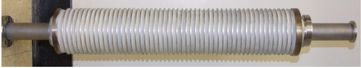
Figure 7. The improved accelerator tube. For this tube, the conductive rings were of inner diameter 3.81 cm and the insulator rings were made with inner diameter of 5.08 cm so as to not allow charge to build up on the walls of the accelerator tube [19].
