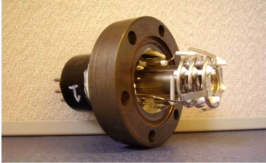
Figure 14. A past design of an electron gun. The filament, cathode can and accelerating grid from a 3RP1 CRT are mounted on a flange with vacuum epoxy so that it can be sealed to the evacuated accelerating tube. Behind the accelerating grid is the cathode can, into which the filament is inserted to heat.
