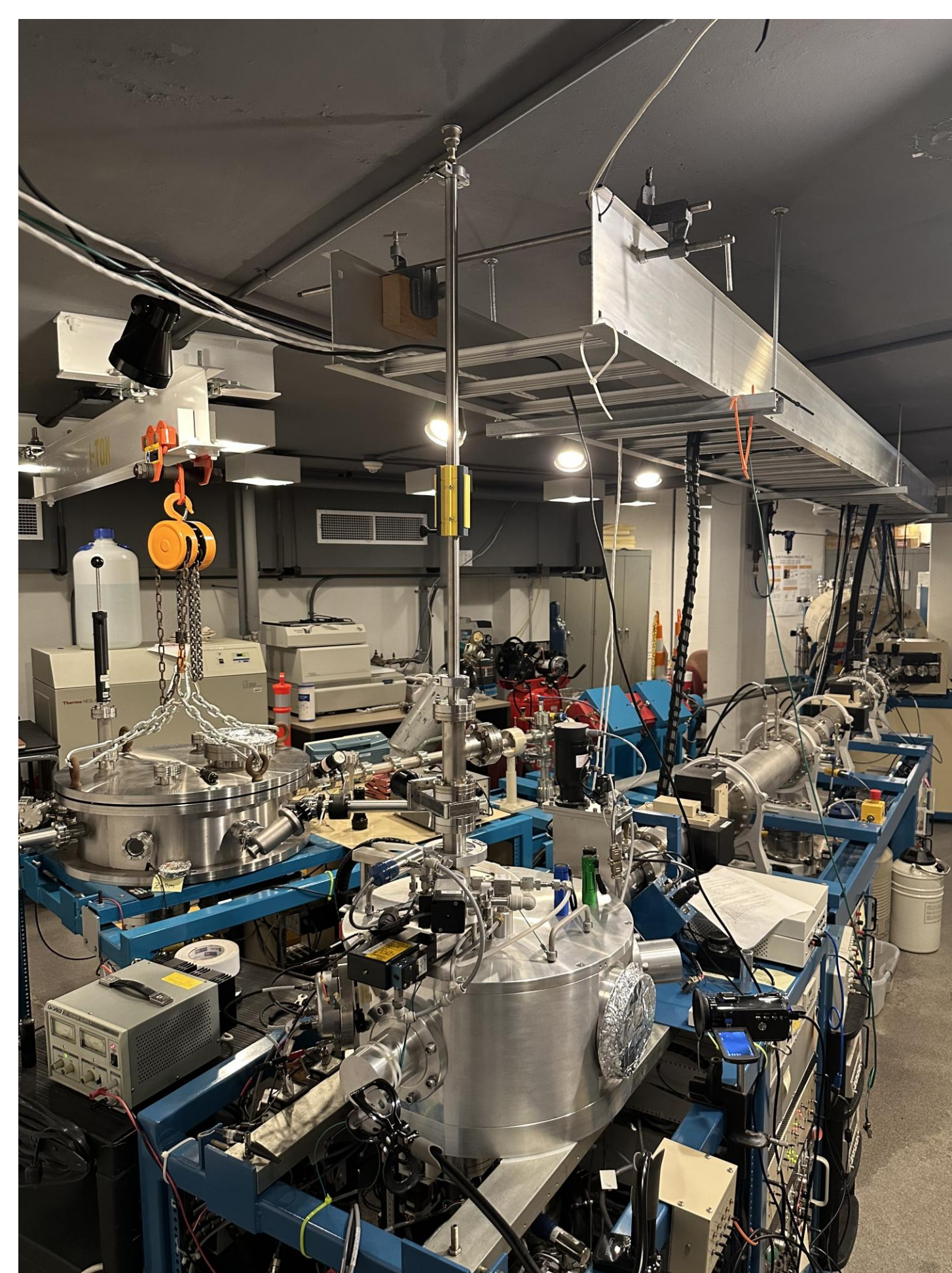
Figure 7 (Upper Right) – The 15R beamline on the 1.7 MV SUNY Geneseo Pelletron. The gate valve and long feedthrough is visible above the scattering chamber lid.
