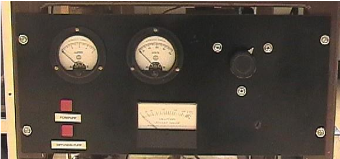
Figure 21. Pictured above are the controls for the vacuum system. The top red button is the fore pump switch and the bottom red button is the diffusion pump switch. The left round gauge is the ammeter, and the round gauge on the right is the voltmeter. The dial on the right side of the panel controls the voltage placed across the heating element. The square gauge indicates the air pressure measured by the piranni gauge.
